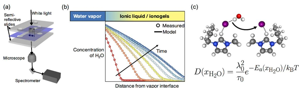
**Figure 1.** (a) Optical train of microfluidic Fabry-Perot interferometry; (b) mFPI enables label-free measurement of concentration gradient-driven diffusion; (c) Diffusion of water in ILs and ionogels is modeled as activated hops between acidic moieties.
