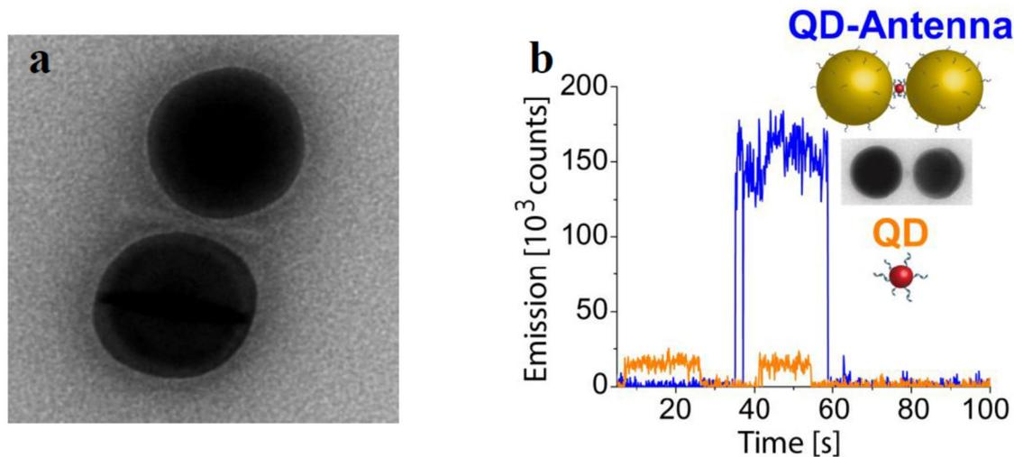
**Figure:** Examples of DNA self-assembled nanoantennas using **a)** a DNA-origami template and **b)** nanocomponents functionalized with complementary DNA sequences. In the latter, an individual QD is positioned between two metallic NPs resulting on enhanced fluorescence emission in respect to individual QDs.
