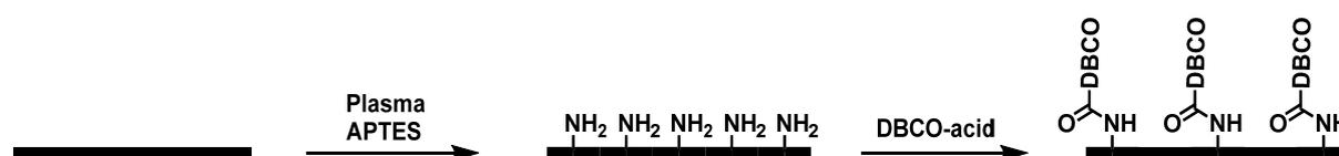
**Figure 2:** Schematic representation of the surface functionalization.
