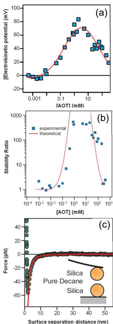
**Figure 1:** Electrokinetic potential of silica in decane as a function of AOT concentration (a), stability ratios in decane as a function of AOT concentration (b), van der Waals interaction measured between two 4  $\mu\text{m}$  silica spheres measured in pure decane (c).
