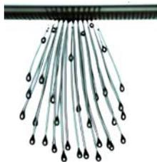
Fig. 1: Shooting yield-stress fluids at screens. At slower speeds, drops cannot penetrate, and the open screen seems closed.
