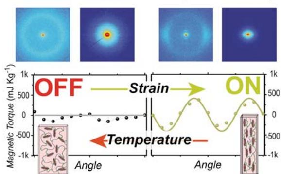
Fig. 1: In the OFF state, 2D X-ray scattering patterns and magnetic torque measurements prove the absence of orientation within the liquid-crystalline elastomer (LCE) nanocomposite. After an applied strain, the oriented ON state is reached and the LCE nanocomposite stores anisotropic magnetic information. This can be released upon heating due to the shape-memory features of the LCE.
