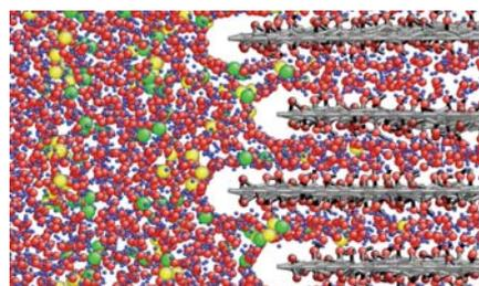
Fig. 2: Graphene oxide with large spacing (1 nm) does not show any ion selectivity.
