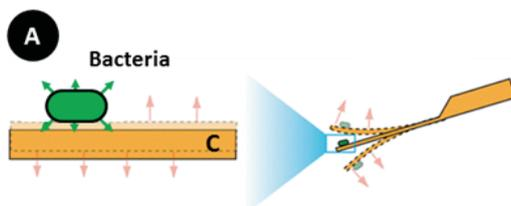
Fig. 1: The nanomotion sensor detects movements of samples deposited on its surface. Bacteria on the sensor's surface cause its fluctuation.
