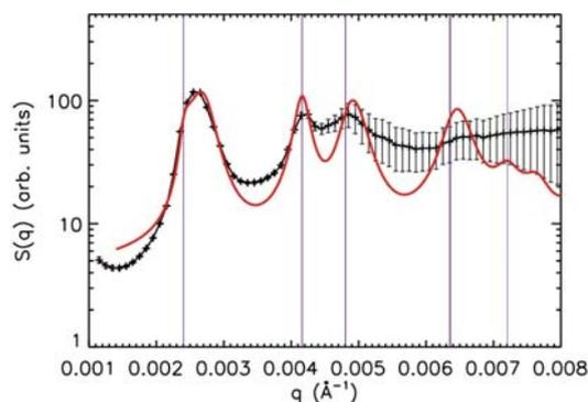
Fig. 1: Structure factor,  $S(q)$ , obtained from SAXS of a sample with volume fraction 0.51. The red line shows the fit to the data obtained with the rhcp structure. The vertical lines show the Bragg peak positions for a hexagonal plane of particles.
