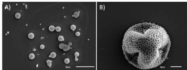
*Fig. 1: Scanning electron micrographs of PBOX-aptamer capsules after cross-linking by irradiation with UV light A) Cross-linkage is performed subsequent to filtration B) large porous structures are observed when no extrusion is performed to reduce the size and fusion of the droplets might occur.*
