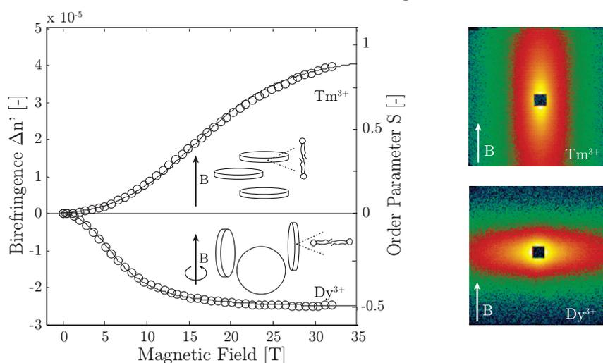
**Figure 1:** Magnetically induced birefringence measurements (left) and SANS measurements in a magnetic field of 8 T (right) showing the different orientation direction of bicelles with  $\text{Tm}^{3+}$  and  $\text{Dy}^{3+}$  [2].
