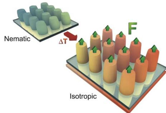
Fig. 1: Micropushers obtained by uniaxial compression with actuation temperatures around 55 °C.
