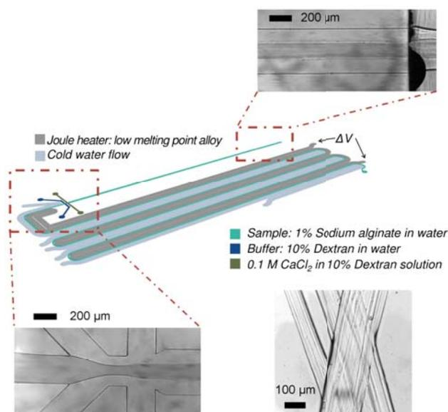
Fig. 1: microfluidic fabrication of calcium alginate soft material with intrinsic concentration gradient. Bottom right: optical image of a sample collected.
