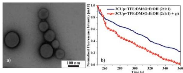
Fig. 1: a) TEM micrograph of pyranine-encapsulated polymersomes; b) Time-driven fluorescence quenching induced by proton diffusion through gA channels inserted inside the polymer membrane vesicles.
