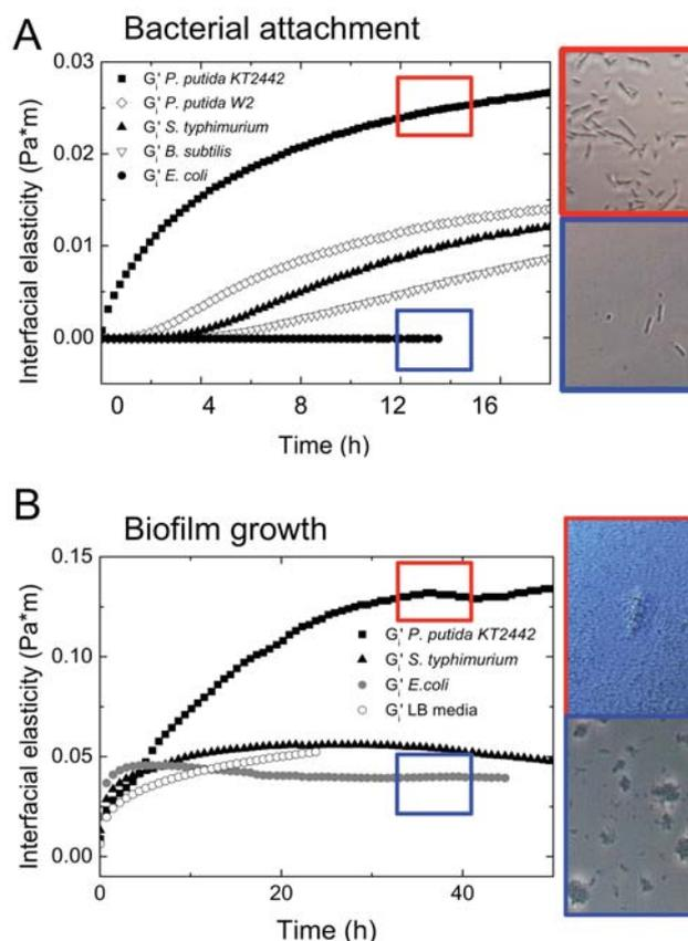
Fig. 1: A: Interfacial rheological time sweep of bacteria adsorbed at the mineral oil-water interface. B: Interfacial rheological time sweep of bacteria adsorbed and growing at the mineral oil-water interface. Microscopic images of the water-oil interface of *E. coli* and *P. putida* KT2442 during bacterial attachment and biofilm growth are shown on the right side.
