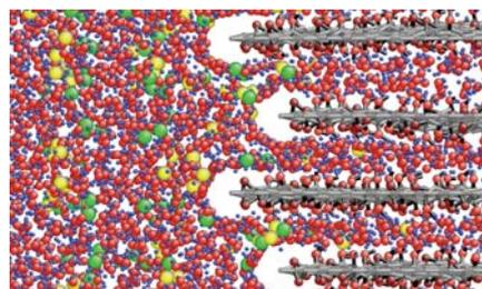
Fig. 1: Small gaps between graphene oxide layers (0.8 nm) let water and Na<sup>+</sup> ions (yellow) pass, while Cl<sup>-</sup> ions (green) are rejected.
