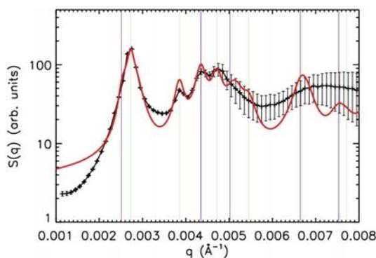
Fig. 2: Structure factor,  $S(q)$ , obtained from SAXS of a sample with volume fraction 0.57. The red line shows the fit to the data obtained with both the rhcp and the bcc structure. The vertical lines show the Bragg peak positions for a hexagonal plane of particles (magenta) and the bcc lattice (green).
