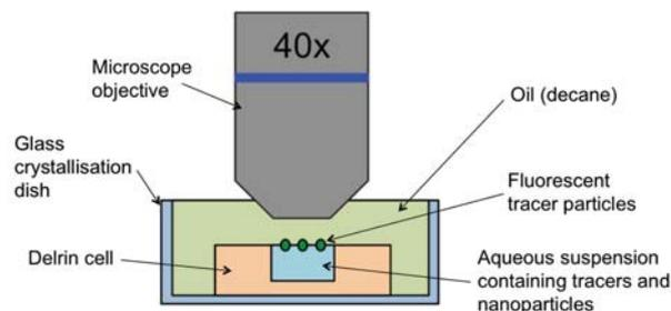
*Fig. 1: Basic setup for microrheology using fluorescence microscopy.*
